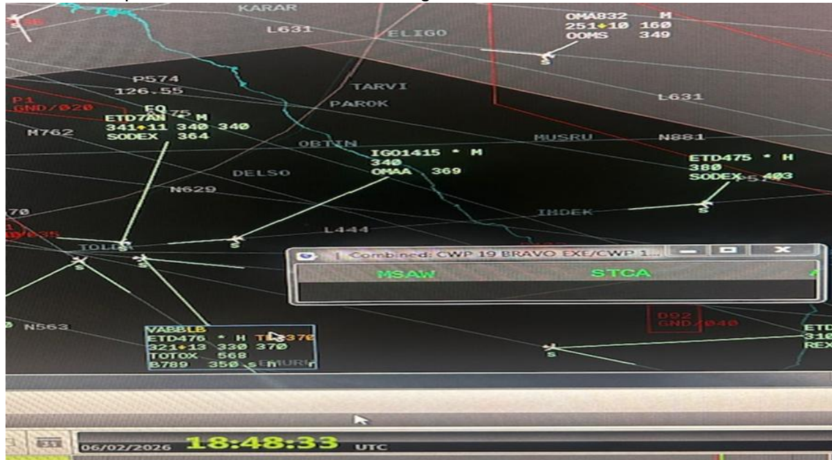
Figure 12 shows conflict display deactivated from the radar screen as both aircraft passed each other (Source: DGAN).
