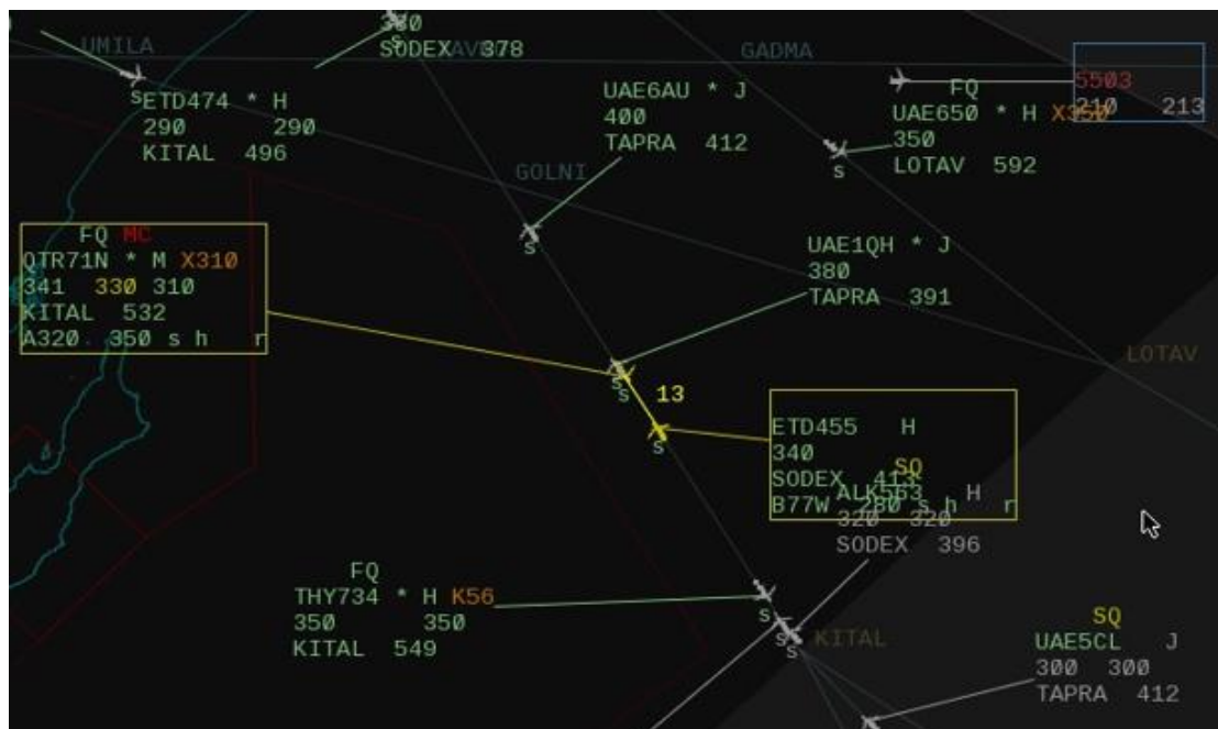
Figure 5: QTR71N at FL341 descending to FL330 and ETD455 at FL340 with a separation of 13 seconds head-on closing rapidly.
