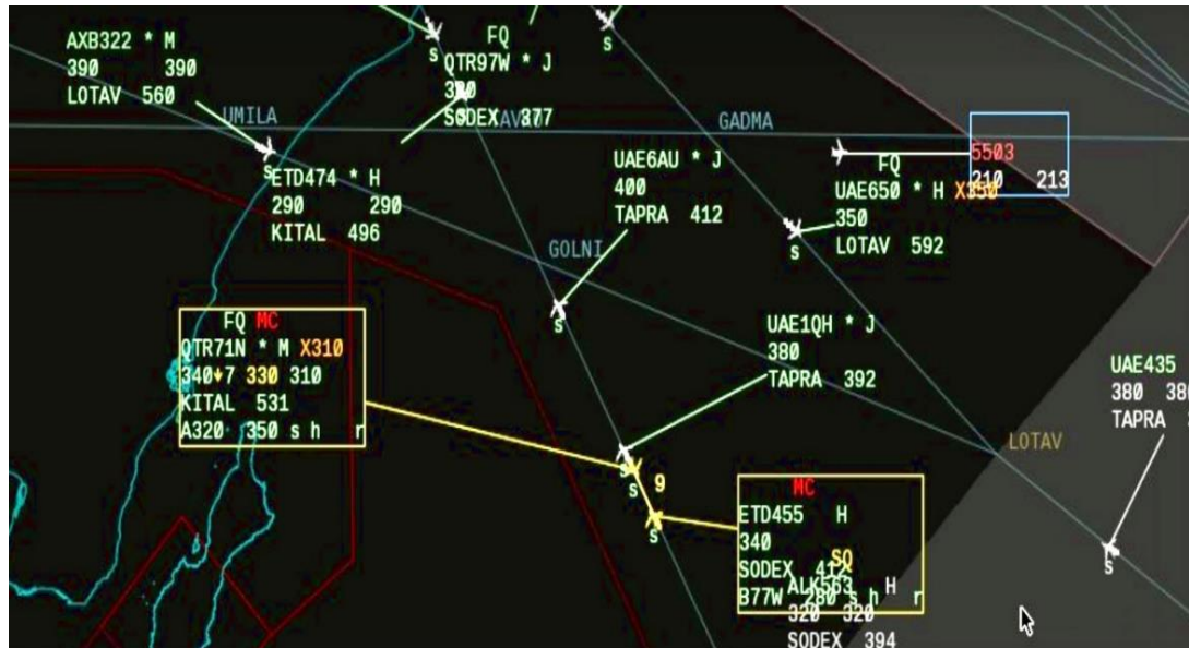
Figure 6 :QTR71N and ETD455 both at FL340, with a distance of 7.38 NM and 9 seconds head-on closing rapidly.
