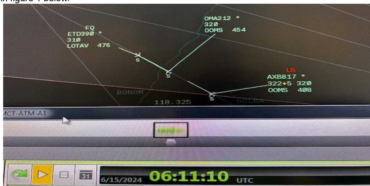
Figure 1: indicating Level Burst (LB) on aircraft AXB817 while descending through FL322 for FL160 with ROD 500FPM.
