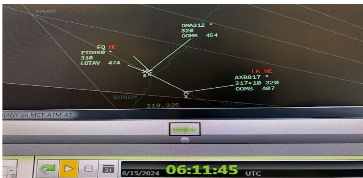
Figure 2: indicates Medium Term Conflict Detection activated on both aircraft ETD390 and aircraft AXB817.
