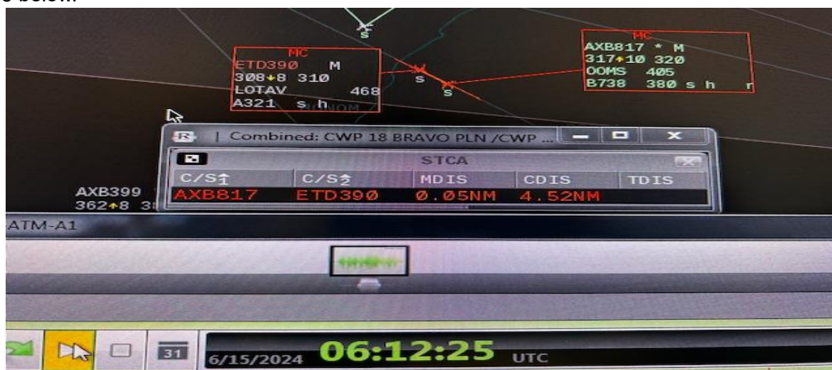
Figure 5: showing aircraft AXB817 while on climb passing through FL317 ROC 1000FPM and aircraft ETD390 on descent passing through FL308 ROD 800FPM with closing distance 4.52NM.
