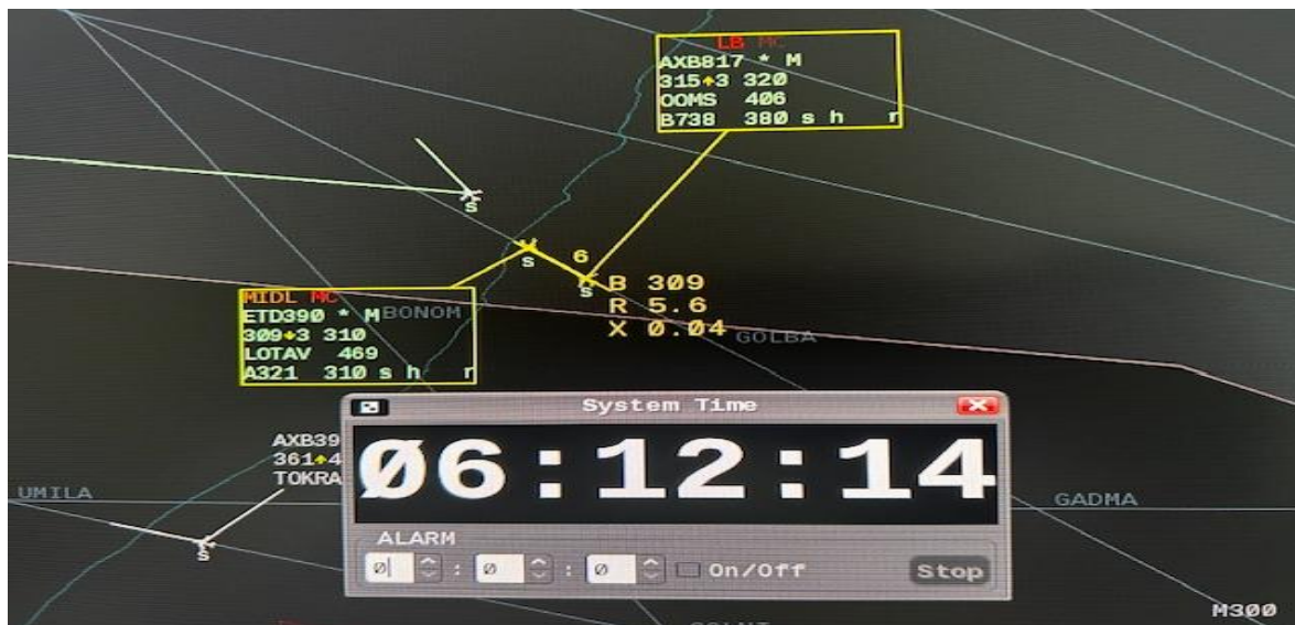
Figure 4: shows aircraft AXB817 was observed on the radar climbing through FL315 to FL320 with ROC 300FPM while aircraft ETD390 was descending through FL309 and leaving FL310 with a ROD 300FPM.
