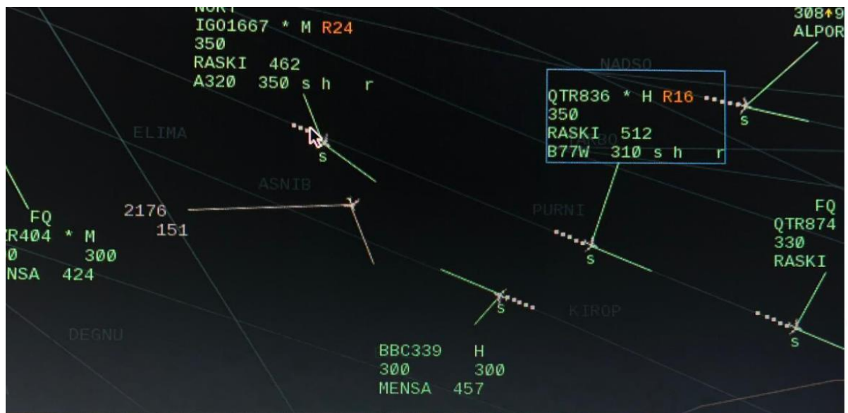
Figure 2. ATC radar screen showing aircraft IGO1667 commencing right turn onto a heading of 150 degrees without ATC clearance.
