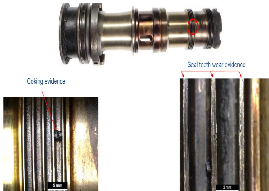
Figure 26. showing abnormal coking at seal teeth location and seal teeth wear
