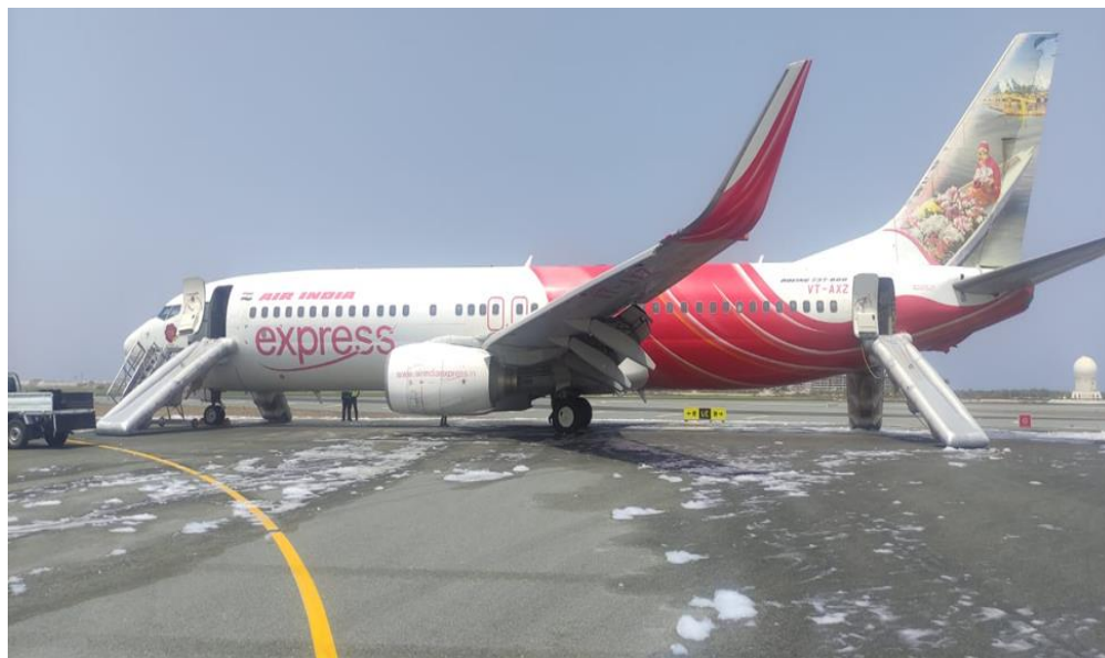
Figure 16 showing the aircraft after it came to a stop with all 4 slides were deployed
