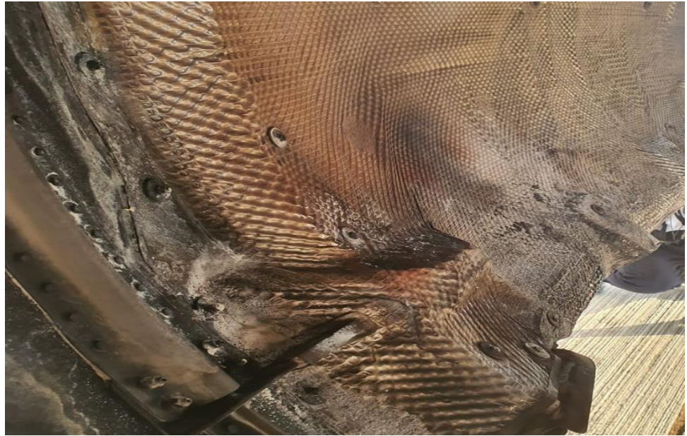
Figure 17 showing the damages to #2 engine thrust reverser thermal blankets
