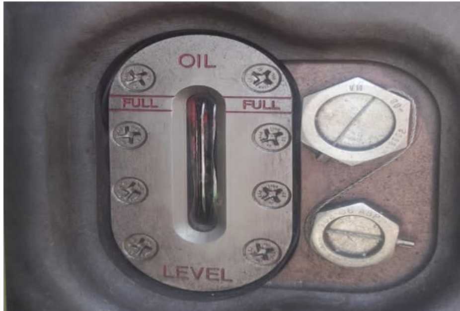
Figure 19 showing the oil level (empty) on the engine 2 sight gauge
