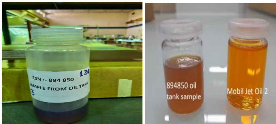
Figure 38. showing the oil sample from oil tank. Figure 28 showing comparisons of the oil sample from oil tank and the Mobil Jet Oil 2
