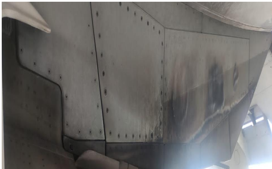
Figure 20. showing the damages to the engine #2 pylon
