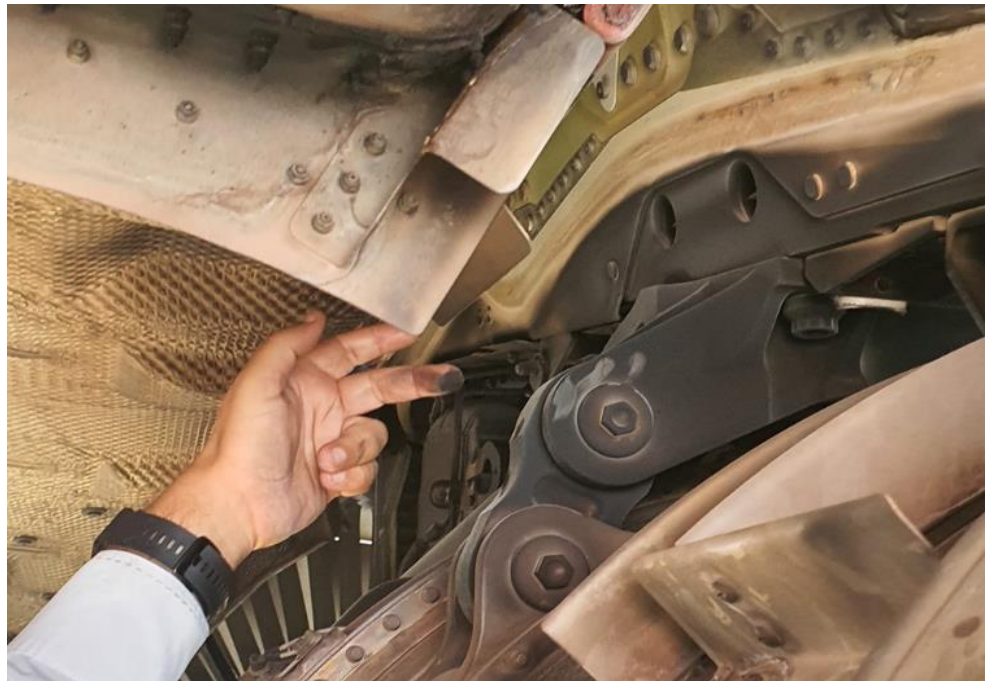
Figure 18 showing damages and soot of the fire
