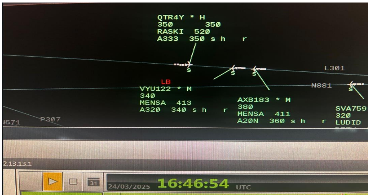
Figure. 1 ATC radar indicating LB activated without any indication of ROC and FL340 on aircraft VYU122 (Source: DGAN)
