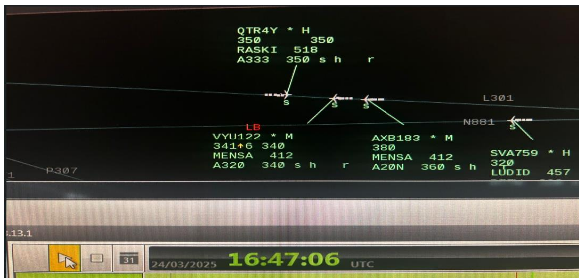
Figure. 2 ATC RDR indicating aircraft VYU122 climbing through FL341 at a ROC of 600FPM (Source: DGAN)
